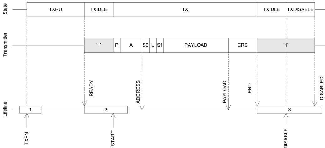
**Figure 5.1:** *The different events generated when the radio transmits a packet. When a packet is received, the same events are generated but with RX instead of TX. Figure is from "nRF52832 Objective Product Specification" [2].*
