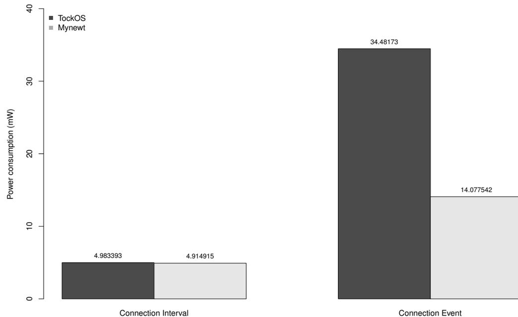
**Figure 6.6:** Bar chart comparing power consumption of Apache Mynewt and TockOS during different events in connection.
