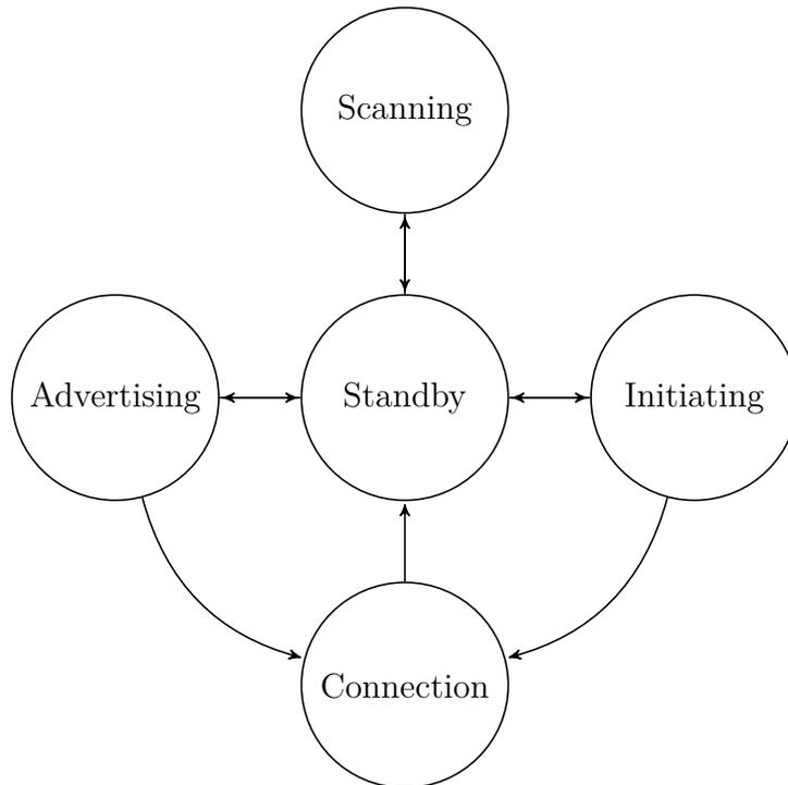
**Figure 2.2:** *Bluetooth Low Energy Link Layer state machine and all the permitted transitions.*
