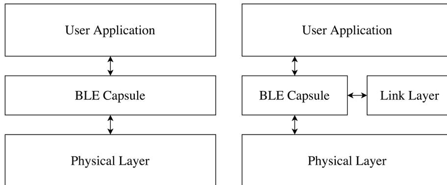
**Figure 4.1:** Comparison of Tock BLE stack before (left) and after (right) our design was implemented.
